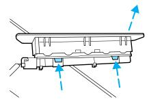
3. Pull the bulb straight out of the socket and push in the new bulb. Install the new bulbs in reverse order.
